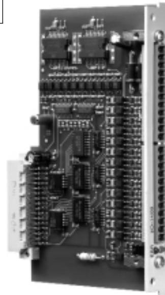
The I/O option card is an extremely economical way of operating servo controllers under position control for simple automation tasks.
