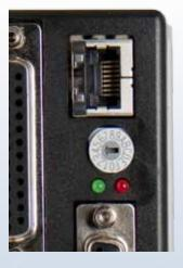
The STAC5 drives come with a rotary switch that can be used to select pre-programmed IP addresses and drive configurations from non-volatile (NV) memory. Each STAC5 drive ships with a predetermined list of 16 IP addresses (including DHCP) and 1 default drive configuration. As your requirements dictate, these 16 rotary switch positions can be customized using the STAC Configurator™ software to define the IP addresses and drive configurations you need for your application.
