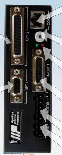
Ethernet port for configuration, programming, and communications.
