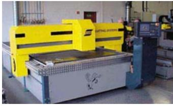
The three-axis gantry plasma cutter was designed to be compact, which left little cabinet space for the controls and servo drives. Another important consideration was price. Since this is a very price competitive industry - especially with smaller machines it was crucial that the selected drive meet the desired price point. The AMC 12A8 servo drive was selected for its high power density and excellent price. The 12A8 provided more than enough performance and fit very well in the cabinet.
